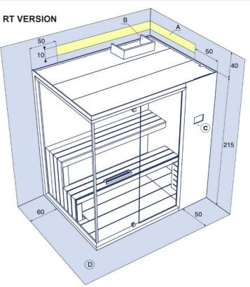
Ghibli Sauna RT corner installation. For LT corner installation the connections are specular
